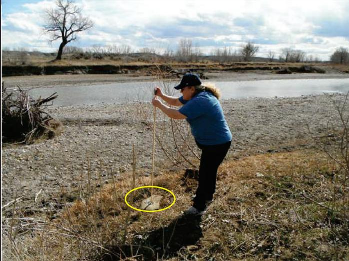
**Figure 1. (top left)** Photographer location on bank. Photographer places a 4 ft. dowel, held plumb, on the rock with the painted circle and points the camera in the direction of the painted arrow to replicate the photo shown in **figure 2.**
