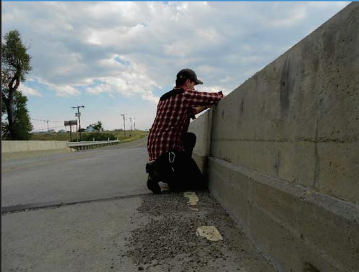
**Figure 1. (top left)** Photographer location and position while taking photo-point photograph. Place the camera in the rectangle painted on the western bridge guardrail facing upstream to replicate the photo shown in **figure 2**.
