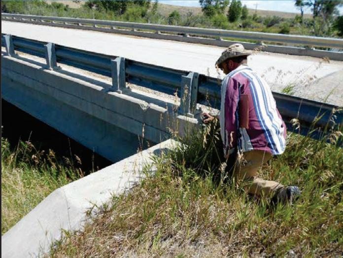
**Figure 1. (top left)** Photographer location and position while taking photo-point photograph. Place the camera facing upstream in the rectangle painted on the southwestern bridge foundation to replicate the photo shown in **figure 2**.
