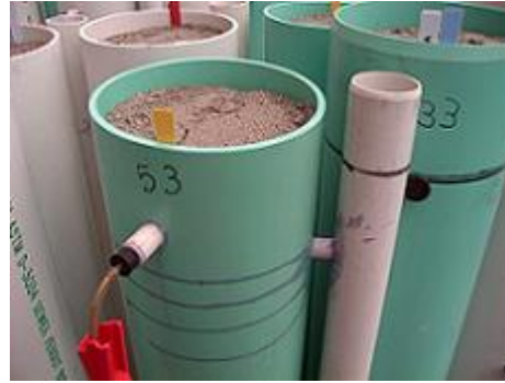
Sampling port at 38 cm water table position.
